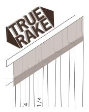
The "rake" of a staircase is the slope, or angle of the stair as it ascends.
