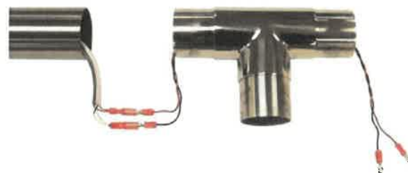
Figure C. Run supplied jumper wires between all fittings, including tees, elbows and 3-way corners. Adjustable fittings and dovetails should already have jumpers installed for your convenience.
