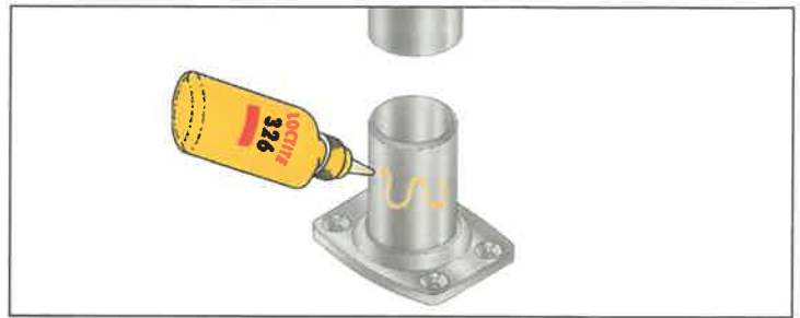
Figure S. Apply a thin bead of Loctite 326 brand adhesive to the bases when you are comfortable that the dry-fit sections are correct.
