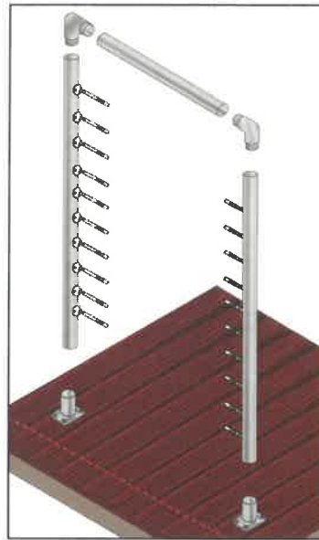
Figure D. (LEFT) Dry-fit each railing section to ensure that everything fits properly. Use a level to make sure that the section is plumb.
