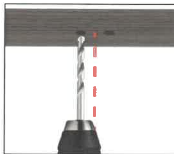
Figure U. (LEFT) Drill pilot holes at the pencil marks in the bottom side of the handrail.
