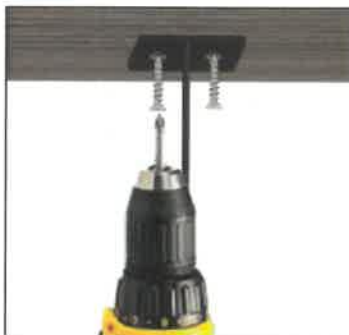
Figure W. (LEFT) Attach the top of the stabilizer to the mounting surface with (2) two #10 x 2" flat head wood screws.
