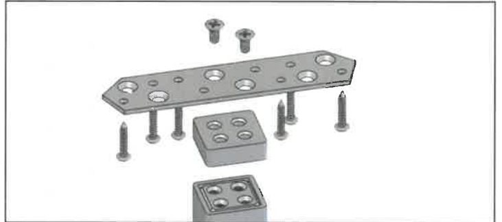
Figure AJ. Attach the spacing block to the post before attaching the top mounting plate.
