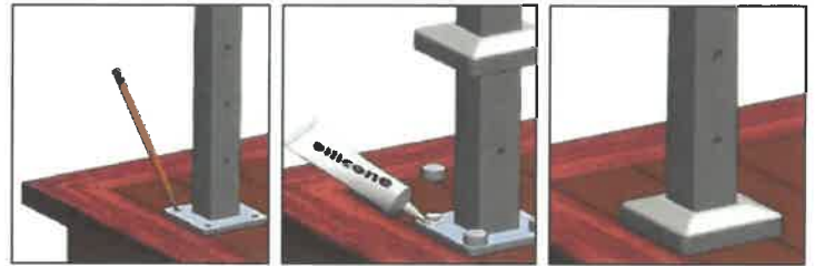
Figure E. (Left) Use the base as a template and mark the four (4) holes for the screws.
