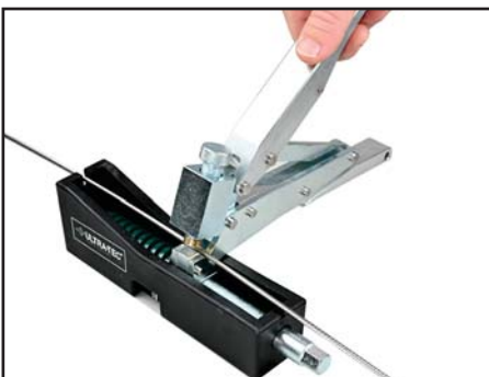
Cable lays into tool
