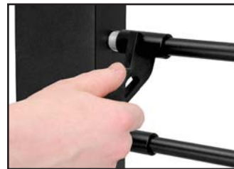
Tighten connector sleeve onto threaded connector
